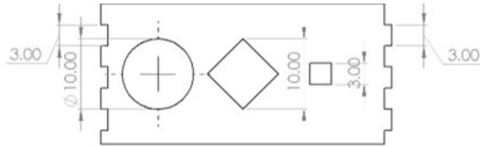
Figure 83: Down-facing features nominal deviation of about 0.18 mm
