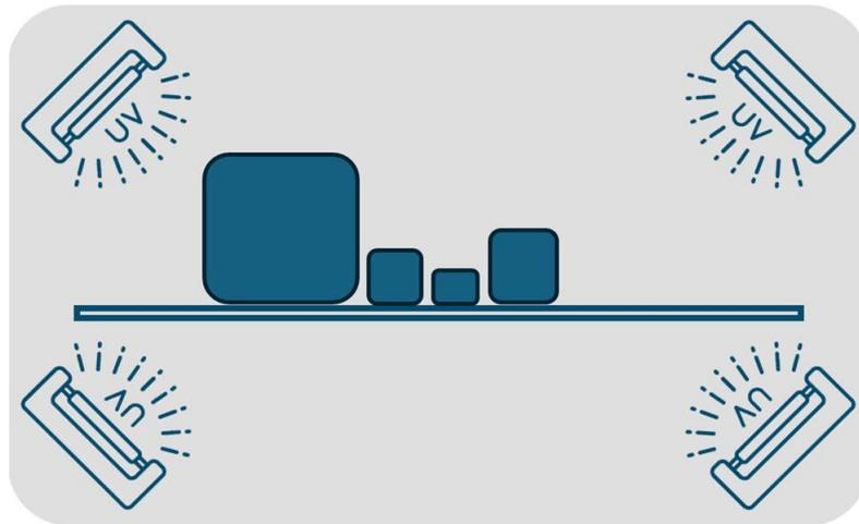
Figure 140: Correct-Parts are spread out and shadowing is minimized
