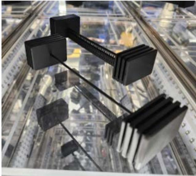
Both models in [Figure 149](#) were printed with the support, but during the curing process one is assisted by the support structure, to keep it from deforming, and the other is cured without the support structure.
