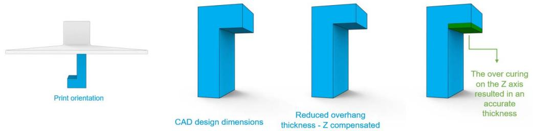
Figure 80: Through cure to optimize the dimensions
