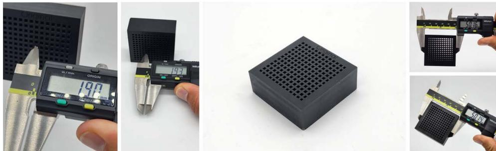
To correct this, we set the edge compensation value to -2, which shifts the surfaces inward by 0.1 mm, effectively enlarging the holes.
