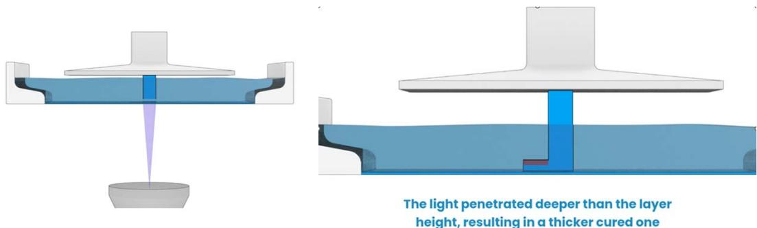
Figure 79: Over-curing on the Z-axis in an accurate thickness
