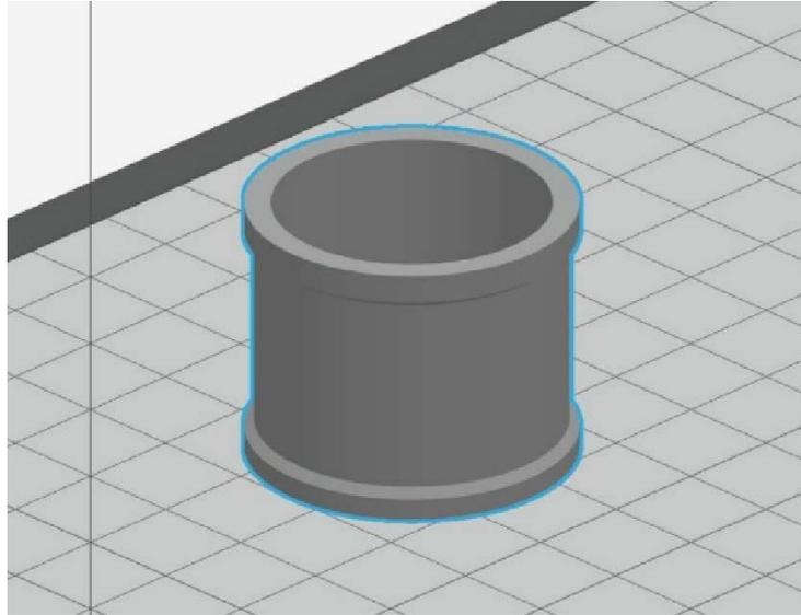
[Figure 135](#) illustrates different *Border Offset* settings. The setting on the right has fewer anchor points and is preferred in this case.
