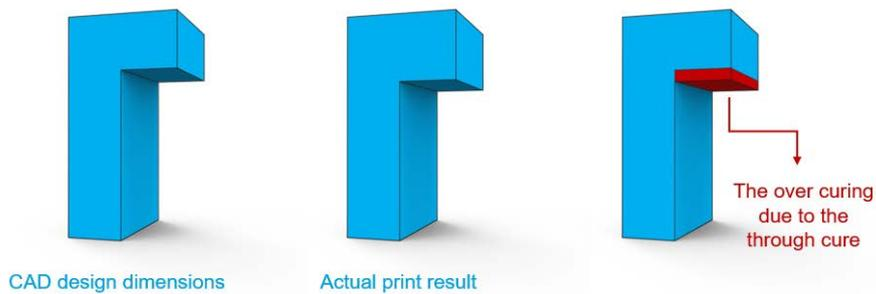
The way to mitigate and compensate for this issue is by reducing the thickness of relevant features and accounting for the extra resin that will cure during the print process. By fine-tuning these parameters, Z compensation ensures each layer is accurately formed, reducing the risk of over-curing and enhancing the accuracy of your 3D prints.
