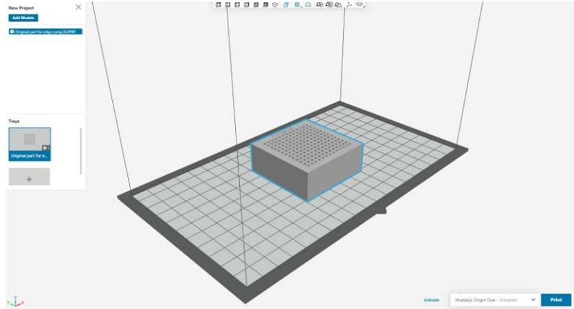
The designed square holes are 2x2 mm, but the actual 3D-printed sizes range is 1.9-1.93 mm.
