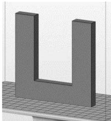
If the orientation can't be changed due to certain constraints, sometimes altering the design will work for removing required supports. The overhang below can be printed without supports by using a chamfer or fillet the overhang.
