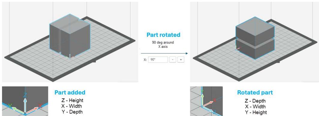
The following examples show the effect of the *Scale* tool on the Z axis for a cube that wasn't rotated compared to one that was rotated:
