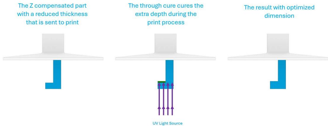
For example, the Loctite IND3172 Cyan material has an expected through-cure value of 0.2 mm. To account for this, we enter the same value in the specified field.
