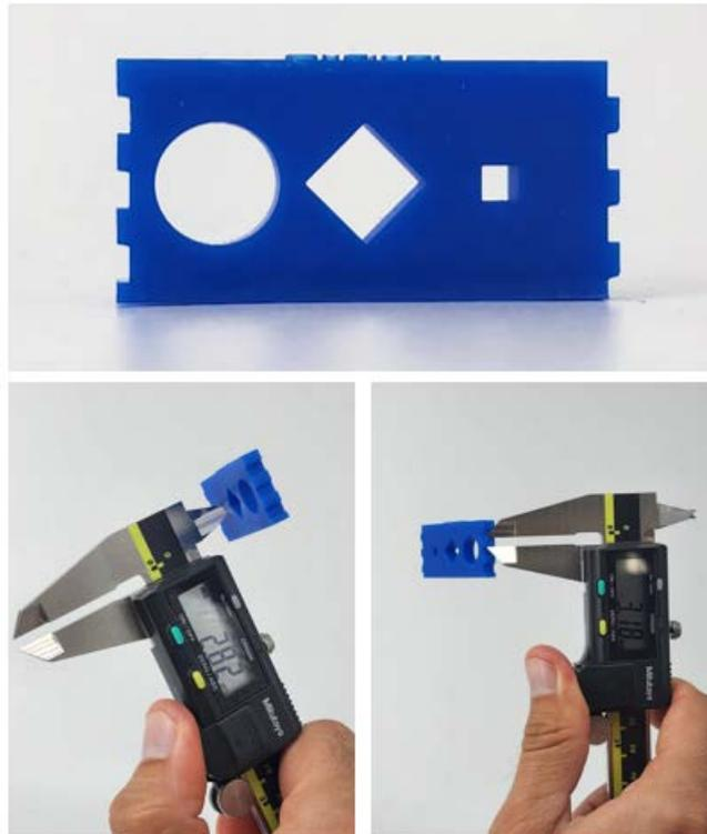
Figure 84: Down-facing features nominal deviation of about 0.03 mm
