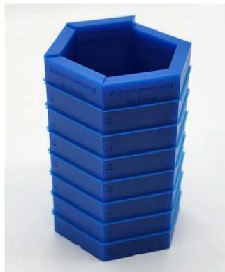
Figure 86: Modified Z-compensated (0.2)—All overhang that are 0.2-mm thick or thinner were gone due to the Z-compensation
