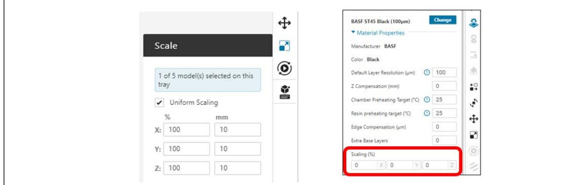
Stratasys-certified material profiles incorporate X, Y, and Z shrinkage compensation factors, but the actual shrinkage varies with different geometries. The *Scaling (%)* option in GrabCAD Print allows you to adjust the scaling factor for the entire job, and then fine tune shrinkage as needed. This tool enables you to:
