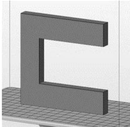
The orientation can be changed so that no supports are required.
