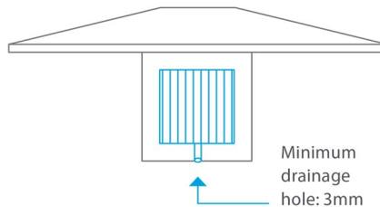
An enclosed volume will not allow resin to escape during the printing process. This will result in a failed build due to uncured resin being trapped in the final part. Create a resin drain hole in all parts with enclosed volumes.
