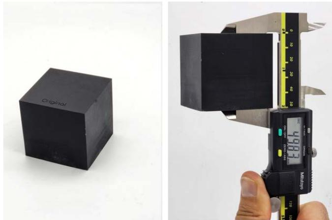
By incorporating two additional base layers, we achieved optimized dimensional accuracy in the Z axis of the printed model.
