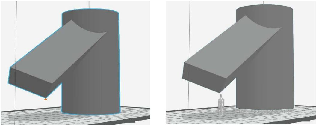
Figure 128: Manually added anchor points (left); improved support structure generated (right)
