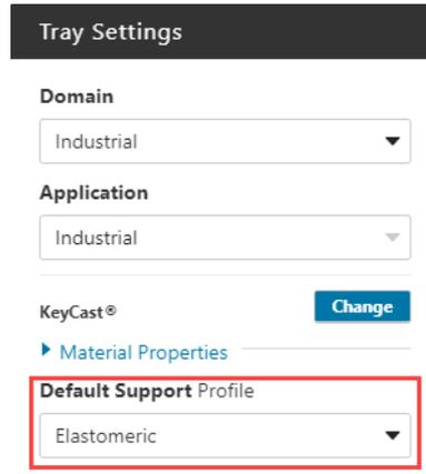
Materials are categorized by their characteristics, which correspond to different support profiles. The recommended support profiles for the Stratasys materials are pre-defined for the listed materials. For information about the recommended support profile that corresponds to the Stratasys-Preferred and Validated materials, see [Table 1](#).
