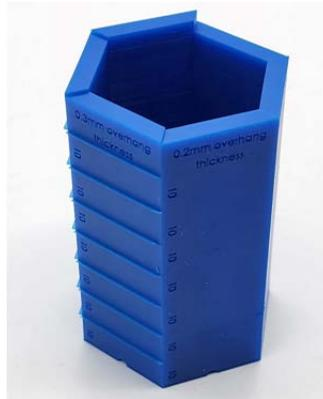
**i** The 0.05-mm thick overhang was not printed on both jobs due to the fact of printing with a 100-µm layer height.
