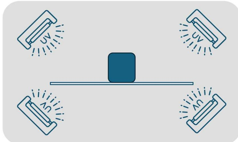
Each material requires a unique UV postcuring process. Some materials require thermal postcuring, as well. You can select a curing program from the 20 programs that are stored on the unit or add new programs, if needed.
